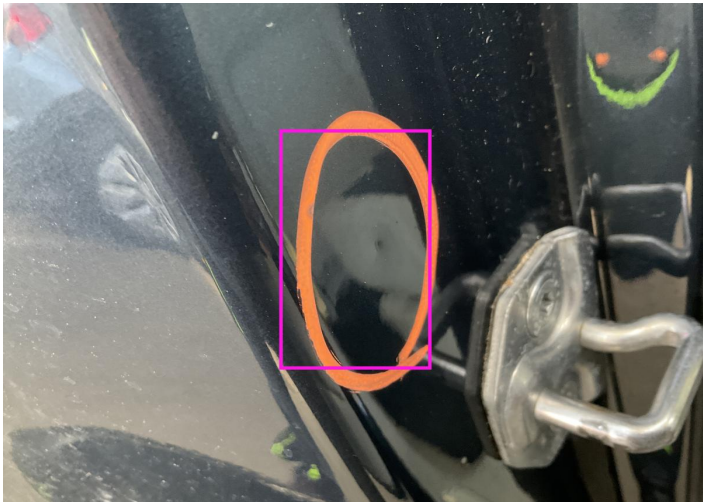
4. Pillar / Back Right Bodywork / Dent / Dent -
