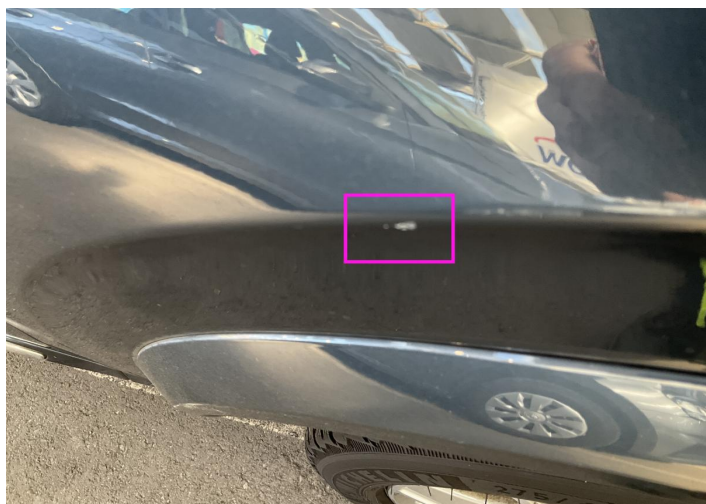
36. Fender / Front Right Paint / Scratch / Scuff -
