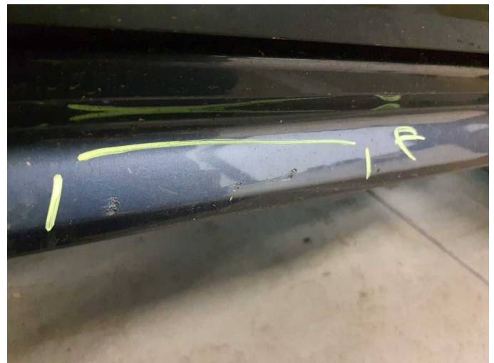
Damage 5: Sill - right side: Trim - Scratched - Smart repair
