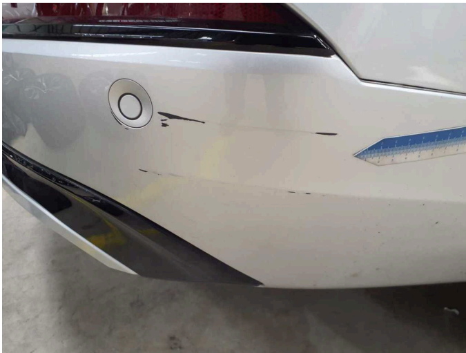
Damage 4: Rear bumper: Rear bumper - Scratch(es) - Paint
