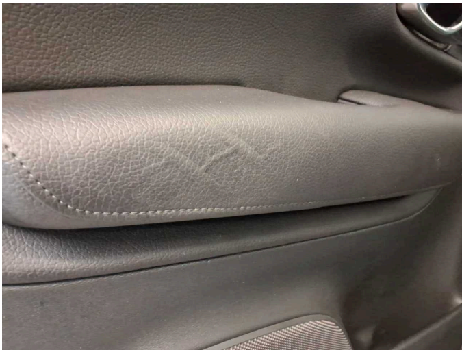
Damage 2: Trim / covers: Door trim - rear left side - Deformed - Smart repair
