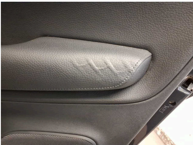
Damage 3: Trim / covers: Door trim - rear right side - Deformed - Smart repair
