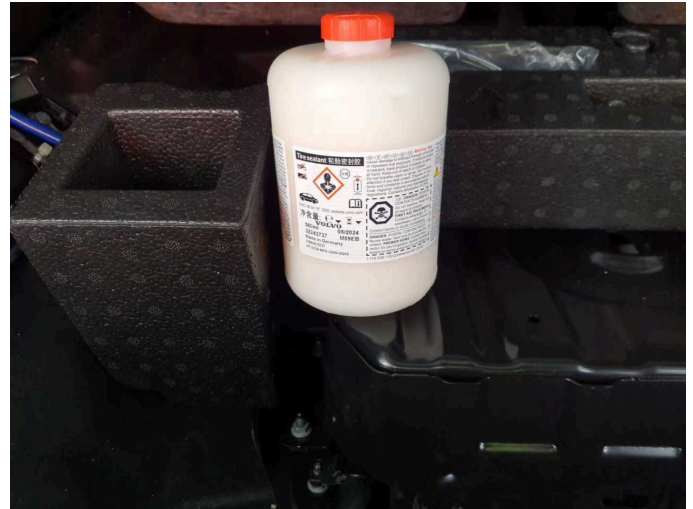
Damage 1: Equipment: Tirefit filler - Expired - Replace
