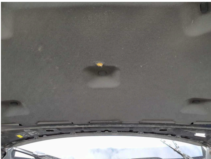
Damage 3: Bonnet: Insulation lining - Damage caused by marten / rodent - Replace
