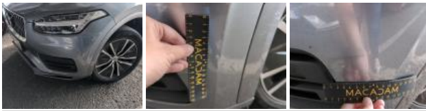
Wing trim FL, Bad repair, Repair and paint (complete)
