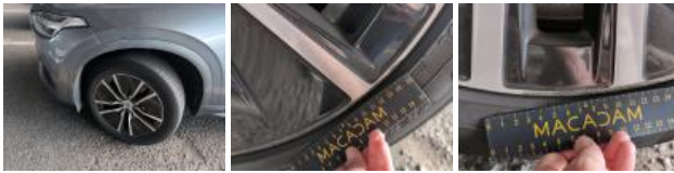
Wing trim RL, Bad repair, Acceptable
