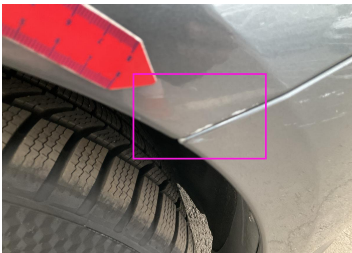
35. Fender / Front Right Paint / Scratch / Scuff -
