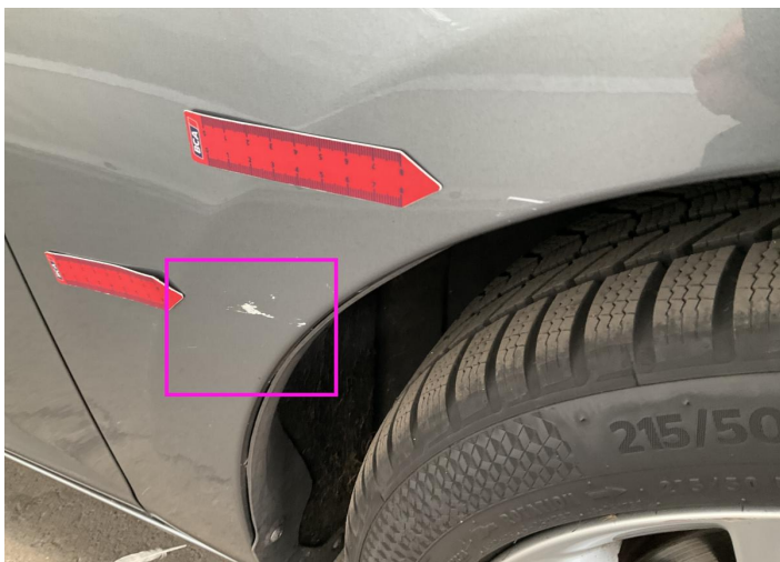
33. Fender / Front Right Paint / Scratch / Scuff -
