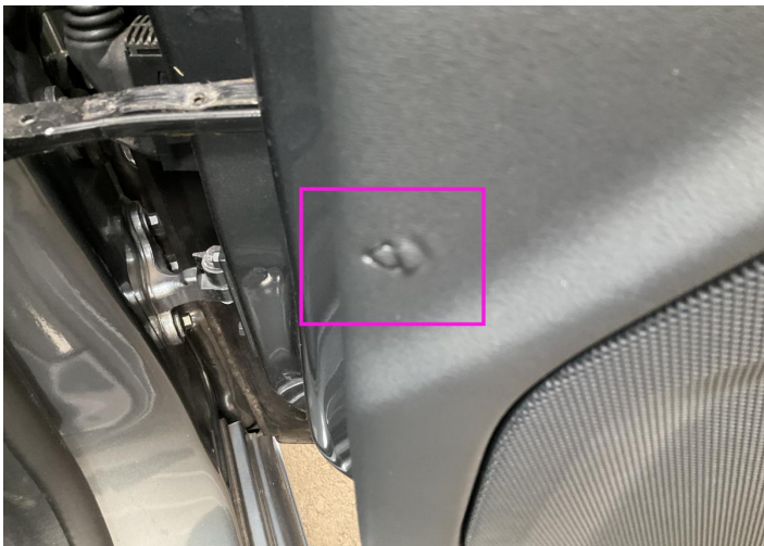
7. Panel Filling / Front Right Interior / Holed -
