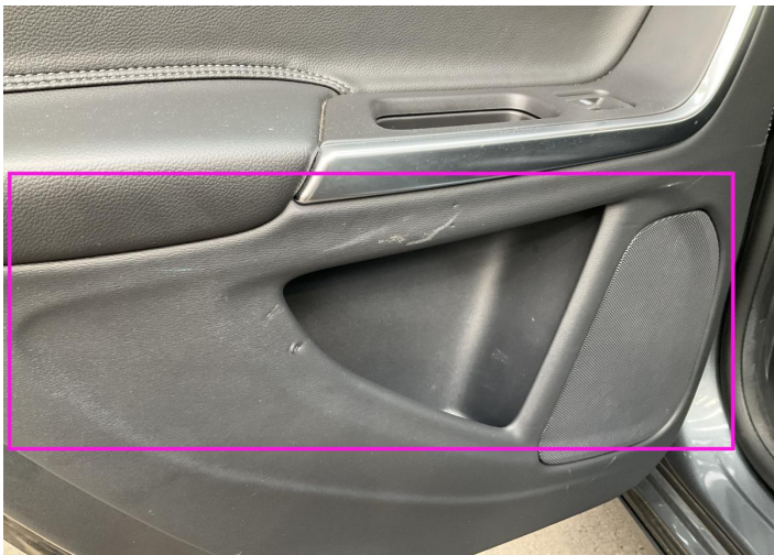
3. Panel Filling / Back Left Interior / Scratched -
