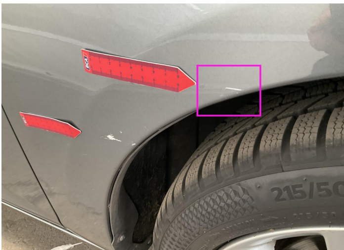
34. Fender / Front Right Paint / Scratch / Scuff -
