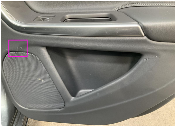
4. Panel Filling / Back Right Interior / Holed -
