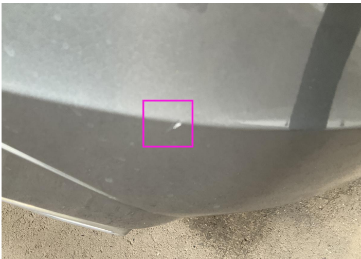
24. Corner Bumper / Back Right Paint / Scratch / Scuff -
