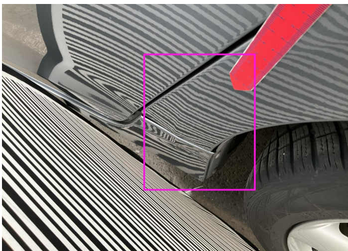
17. Fender / Back Left Bodywork / Dent / Dent -
