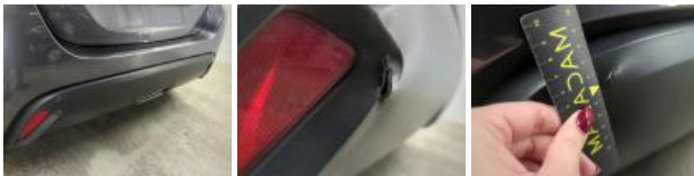
Bumper RM, Broken, Replace
