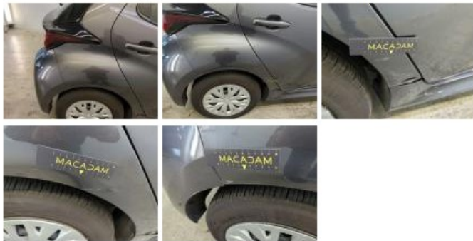
Sill trim R, Scratch(es), Repair and paint (complete)
