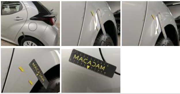
Bumper F, Scratch(es), Repair and paint (complete)
