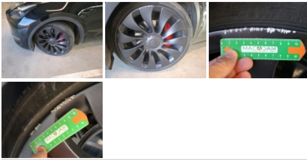
Tyre RL, Out of tolerance, Replace
