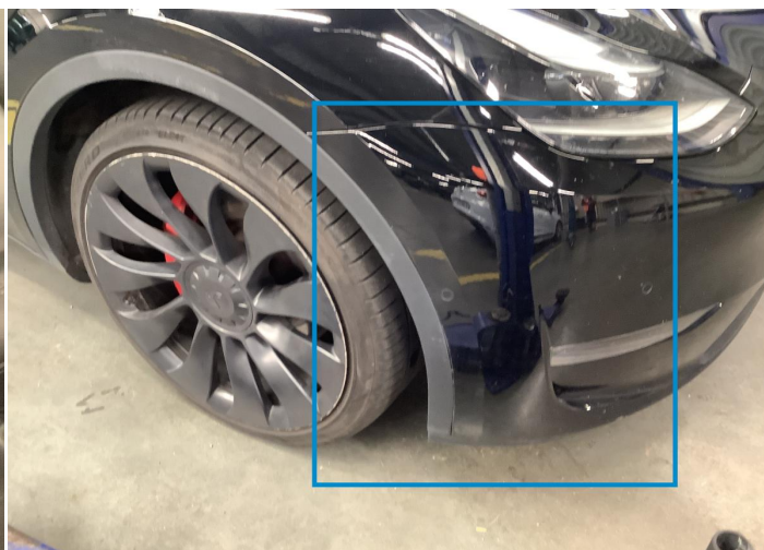
20. Corner Bumper / Front Right Paint / Scratch / Line -
