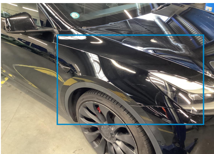
14. Fender / Front Right Paint / Scratch / Line -
