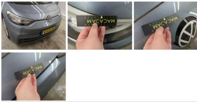
Bumper F, Scratch(es), Repair and paint (complete)
