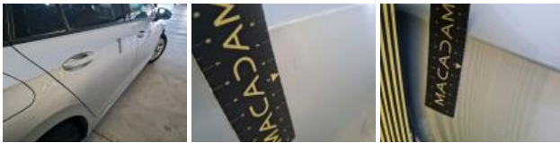
Outside rear-view mirror housing R, Scratch(es), Acceptable
