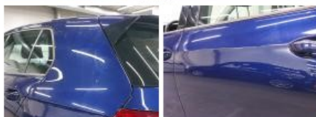
Roof, Dent(s), Acceptable
