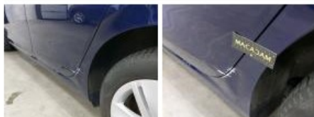
Door RL, Scratch(es), Repair and paint (complete)
