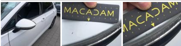
Outside rear-view mirror housing L, Scratch(es), Repair and paint (complete)
