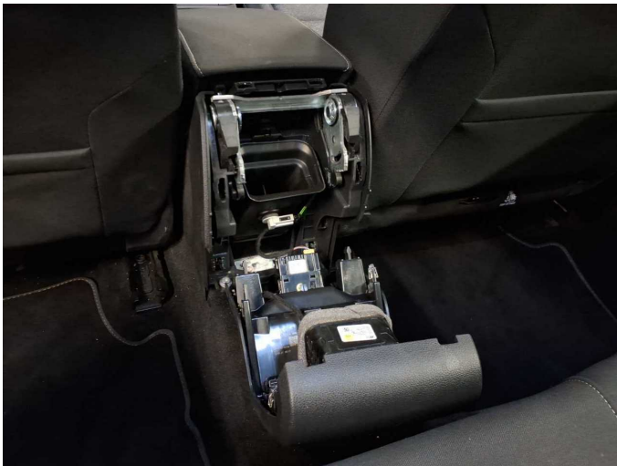
Damage 7: Instrument panel: Centre console - rear - Broken / torn - Replace
