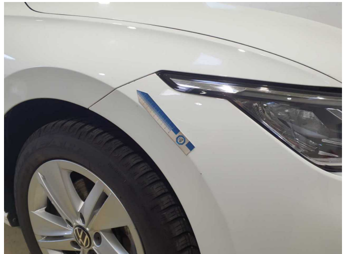
Damage 7: Front bumper: Front bumper - Scratched - Paint
