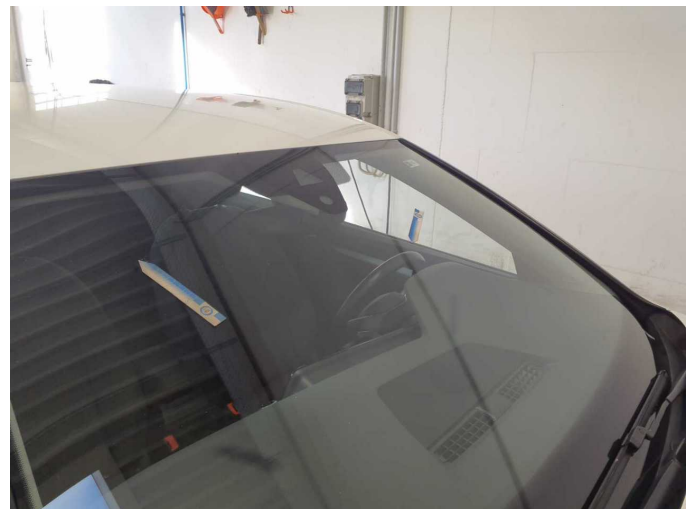
Wear and tear 1: Vehicle glazing: Windscreen with lane departure assistant (ohne Rissbildung) - Stone chips - No deduction
