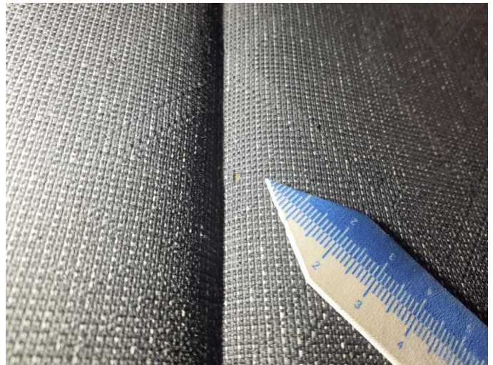
Damage 4: Seat - front: Seat cover - left side - Burn hole (cigarettes) - Smart repair
