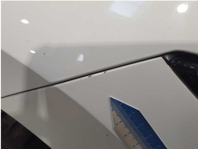
Damage 7: Front bumper: Front bumper - Scratched - Paint
