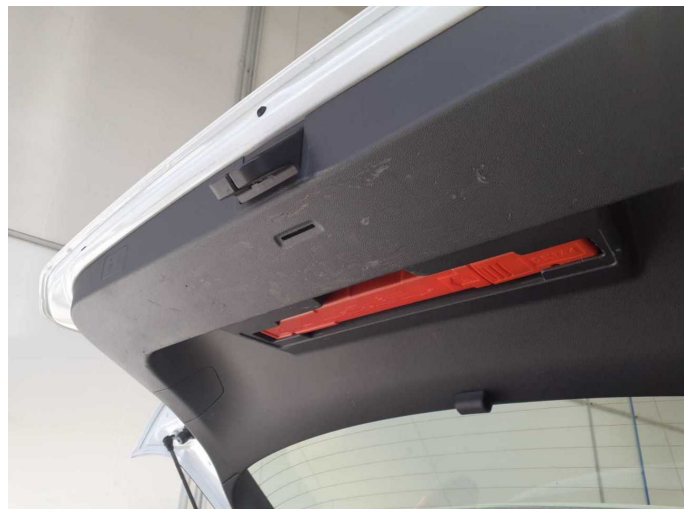
Damage 5: Boot lid / rear door: Trim - standard - lower - Scratched - Replace
