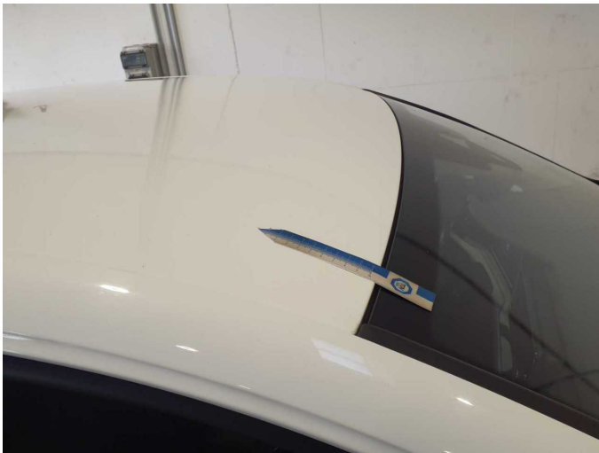
Damage 8: Roof: Roof - Corrosion - Repair and paint
