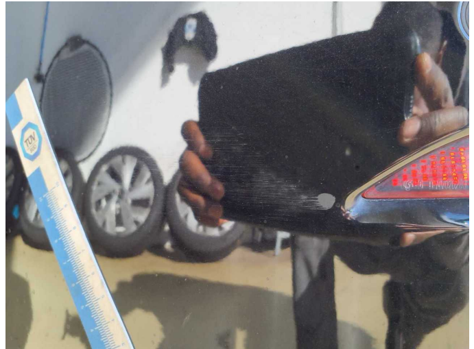
Damage 8: Rear bumper: Rear bumper - Scratch(es) - Paint
