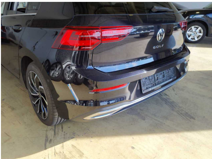
Damage 8: Rear bumper: Rear bumper - Scratch(es) - Paint
