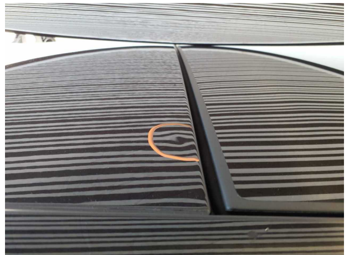
Damage 2: Roof: Roof - dent(s) - Smart repair
