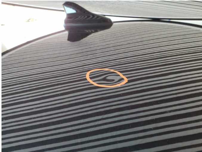
Damage 2: Roof: Roof - dent(s) - Smart repair
