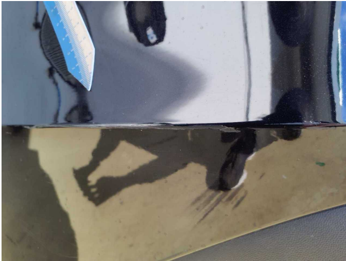
Damage 8: Rear bumper: Rear bumper - Scratch(es) - Paint
