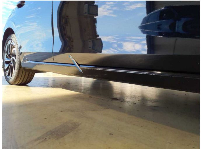
Damage 4: Sill - right side: Sill - Deformed - Smart repair
