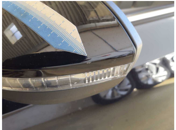
Wear and tear 1: Wing mirror - left side: Cap - Scratch(es) - No deduction
