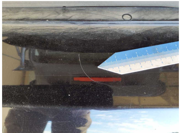
Damage 8: Rear bumper: Rear bumper - Scratch(es) - Paint
