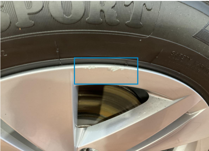
1. Rim / Front Left Paint / Stone Chip -
