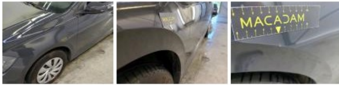
Door RL, Scratch(es), Repair and paint (complete)
