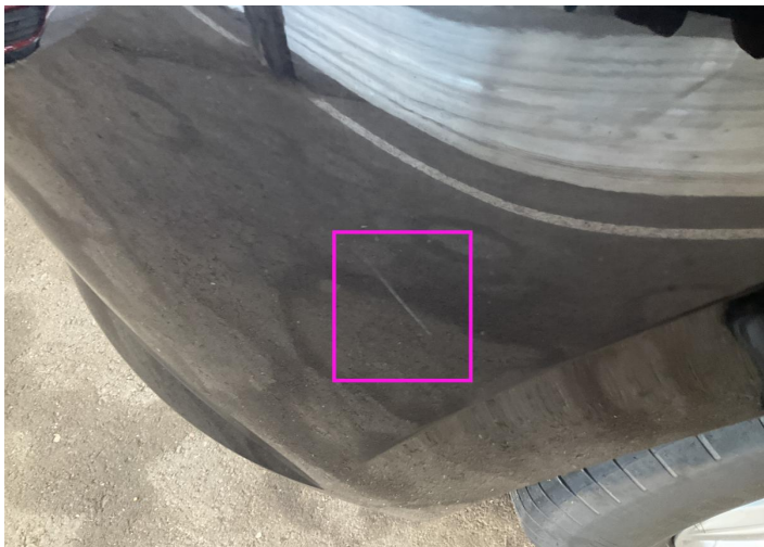
9. Corner Bumper / Back Right Paint / Scratch / Scuff -
