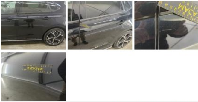
Wing RL, Dent(s) and scratch(es), Repair and paint (complete)
