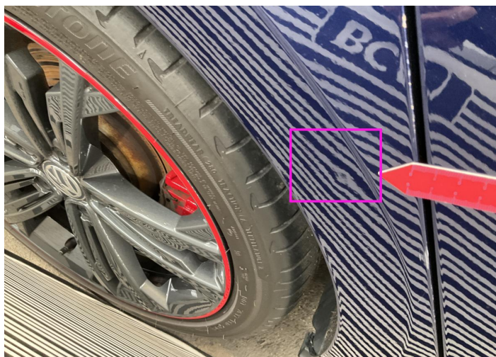
7. Side Panel / Back Right Bodywork / Dent / Dent -
