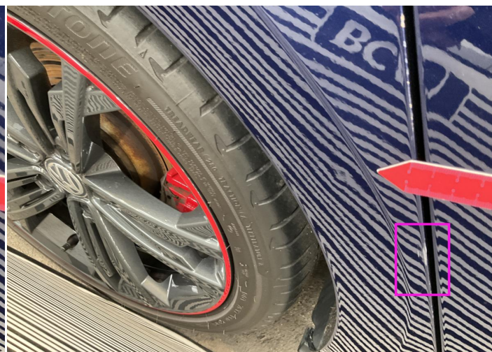
8. Side Panel / Back Right Paint / Scratch / Scuff -
