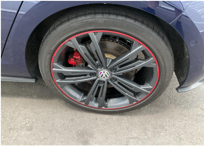
4. Rim / Back Left Out of Bodywork / Scratch -
