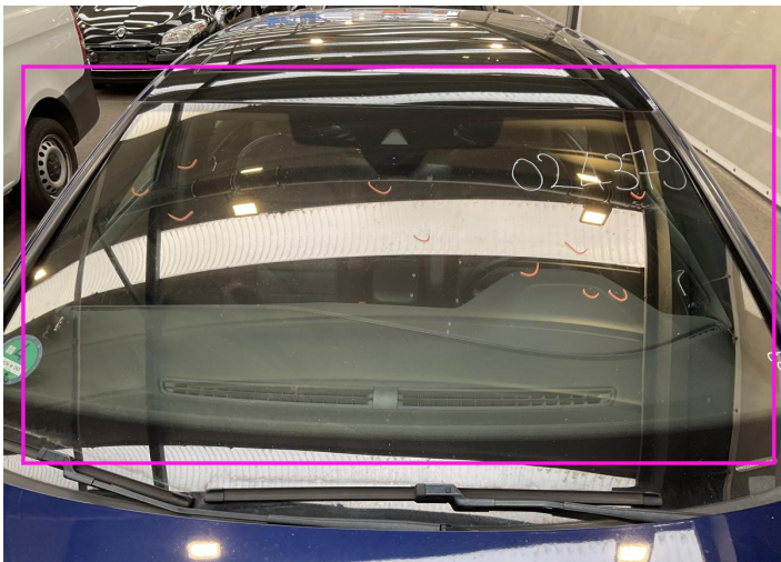
1. Windshield / Front Paint / Chipping -
