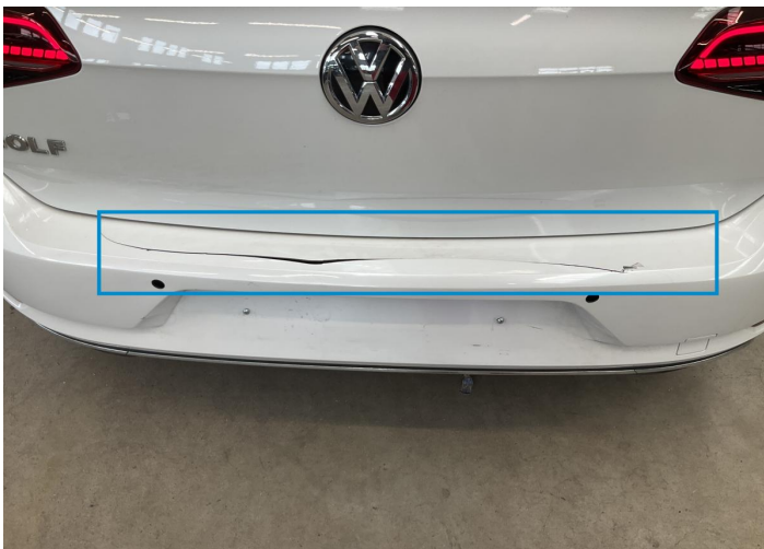
6. Bumper / Back Bodywork / Breakage / Crack -
