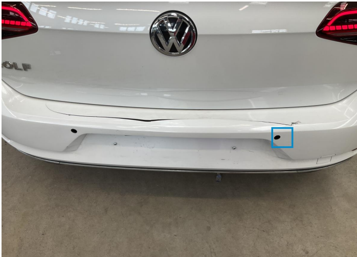
7. Bumper / Back Missing Part -
