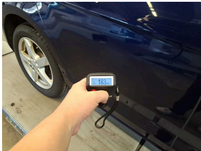
Repainting 2: Door - rear right side, Door - front right side
