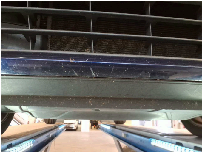
Damage 3: Front bumper: Front bumper - Scratched - Paint
