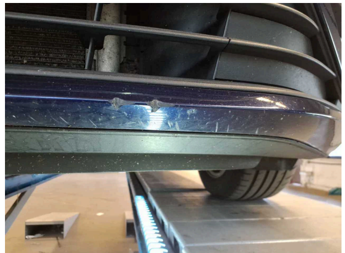
Damage 3: Front bumper: Front bumper - Scratched - Paint
