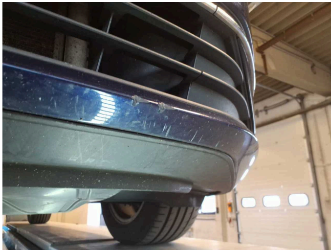
Damage 3: Front bumper: Front bumper - Scratched - Paint
