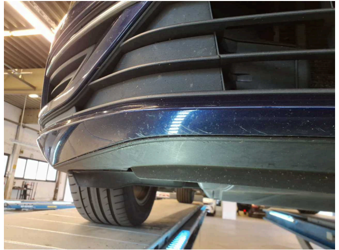
Damage 3: Front bumper: Front bumper - Scratched - Paint
