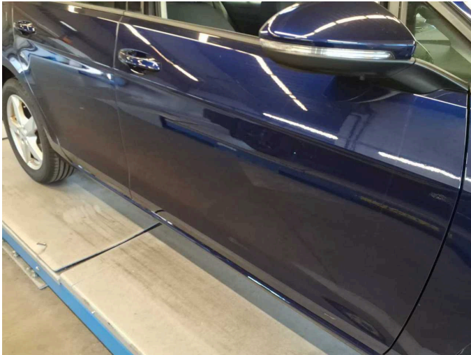
Damage 5: Door - front right side: Door ("Orangenhaut" erkennbar) - Unprofessionally repaired - Repair and paint
