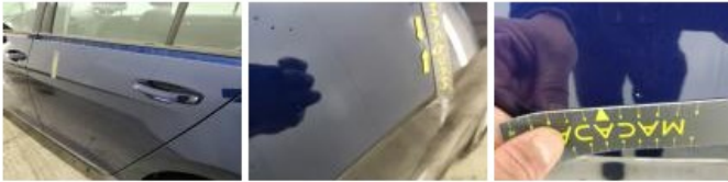
Door FL, Scratch(es), Repair and paint (complete)
