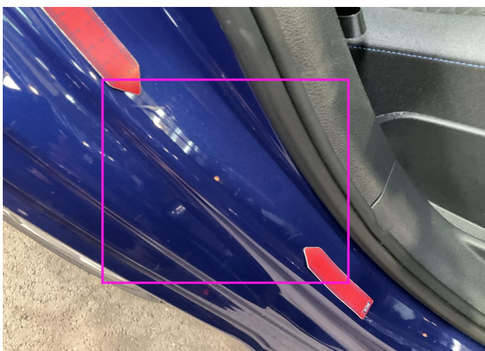
3. Pillar / Back Right Paint / Scratch / Scuff -
