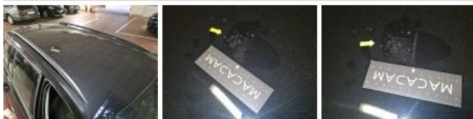
Roof, Chemical polution, Repair and paint (complete)
