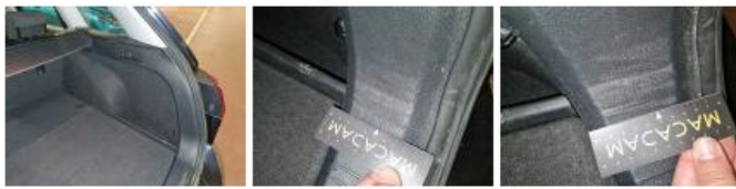
Interior covering C pillar R, Scratch(es), Acceptable
