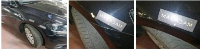
Wing RR, Dent(s), Paintless dent repair
