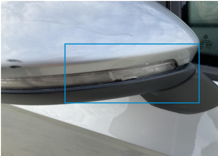
4. Mirror Repeater / Right Bodywork / Breakage -
