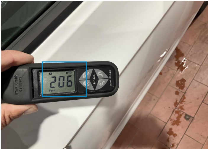
3. Door / Front Right Paint / Poor Previous Repair -
