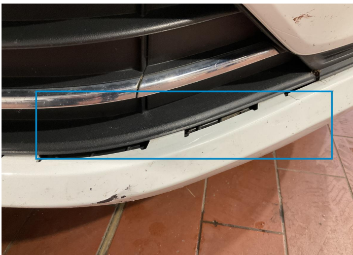
10. Grille / Front Bodywork / Breakage / Hole -
