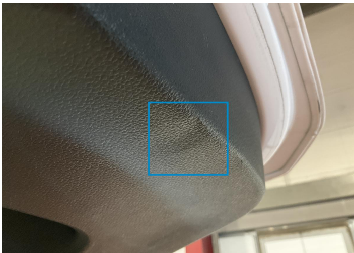
1. Tailgate Upholstery / Back Interior / Dented -
