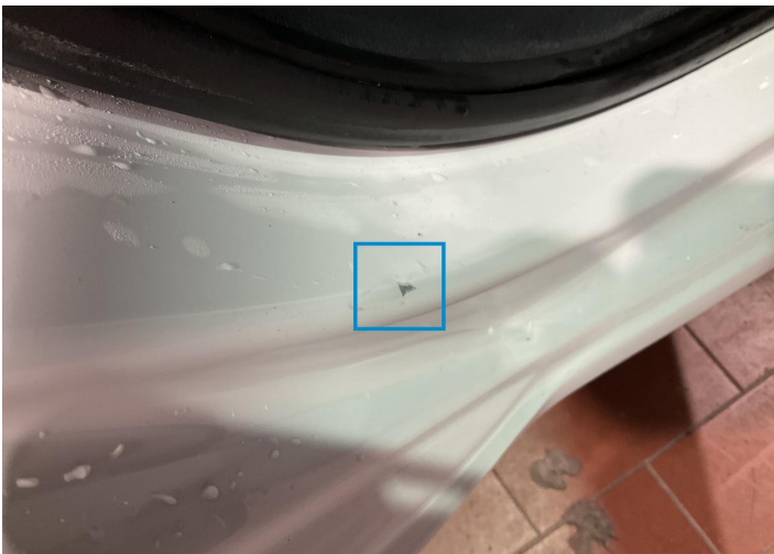
2. Pillar / Back Right Bodywork / Dent / Dent -
