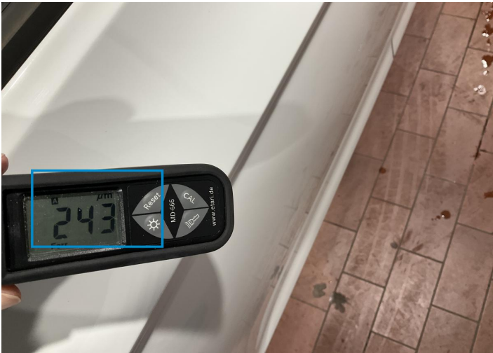
4. Door / Back Right Paint / Poor Previous Repair -
