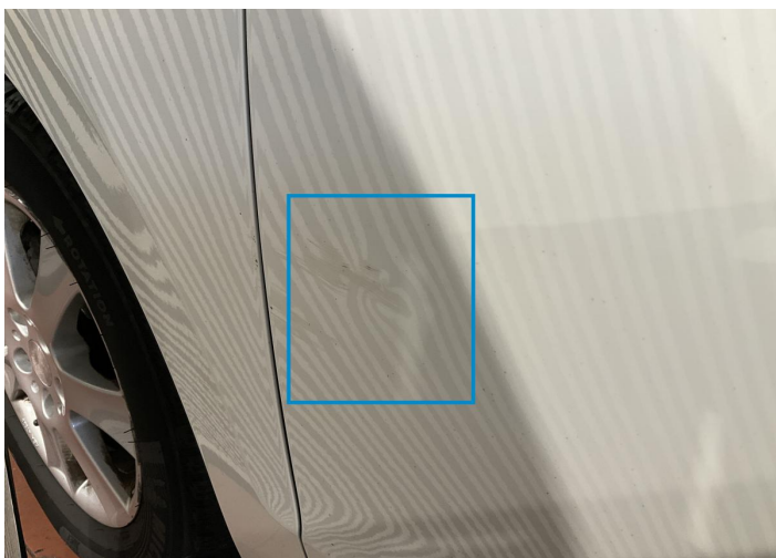
7. Door / Front Left Bodywork / Dent / Dent -
