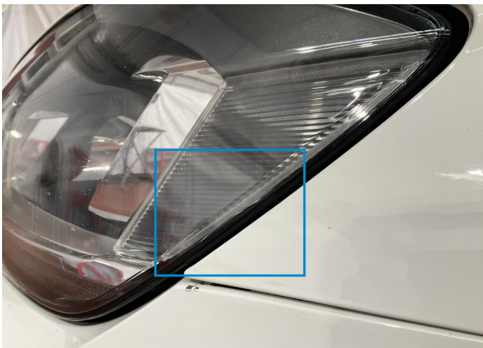
18. Front Light / Front Left Glass Break -
