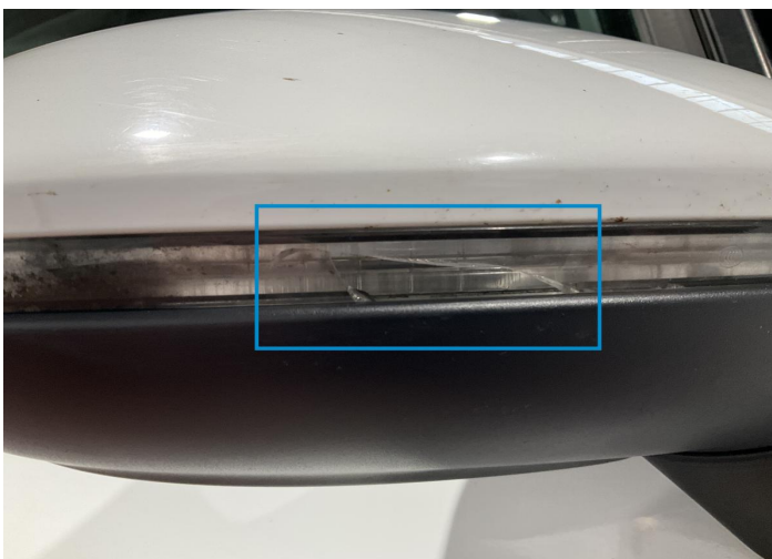
12. Mirror Repeater / Right Bodywork / Breakage / Crack -
