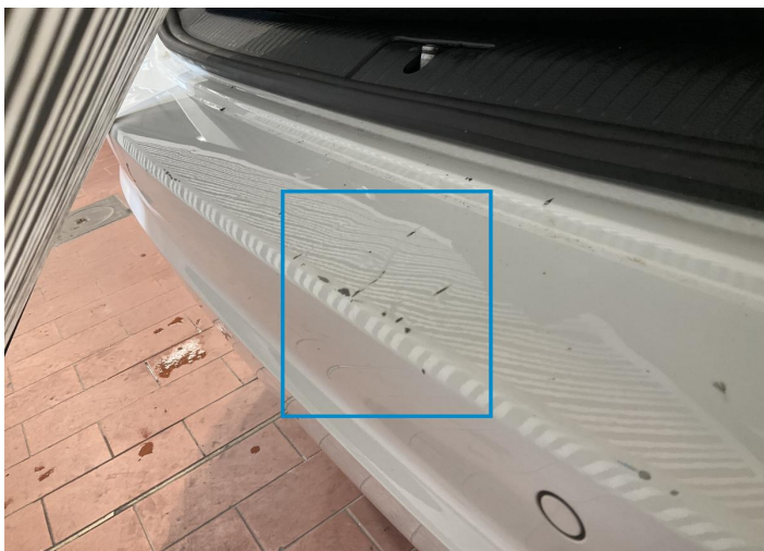
15. Bumper / Back Bodywork / Dent / Dent -
