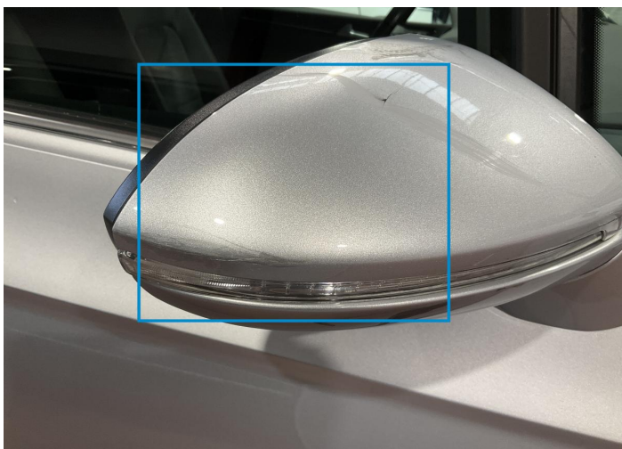
5. Mirror / Front Right Bodywork / Breakage / Crack -
