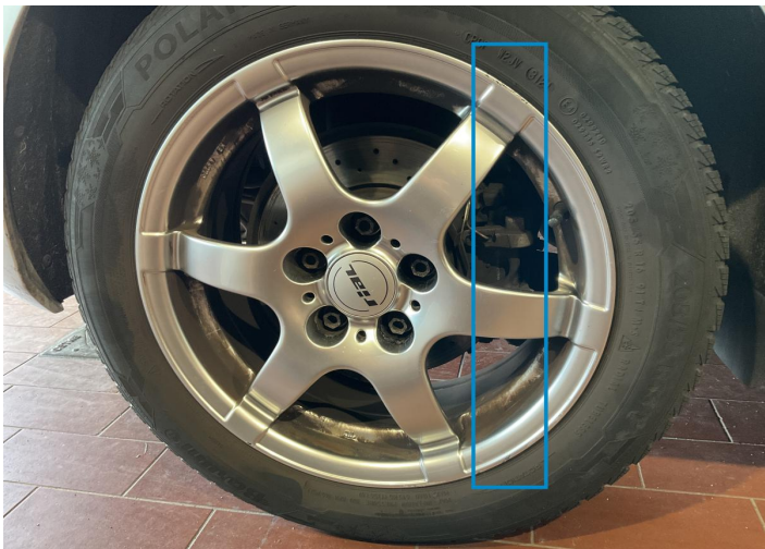
9. Rim / Back Right Out of Bodywork / Scratch -
