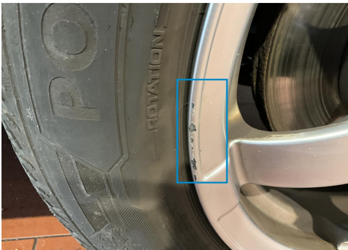
12. Rim / Front Right Out of Bodywork / Scratch -
