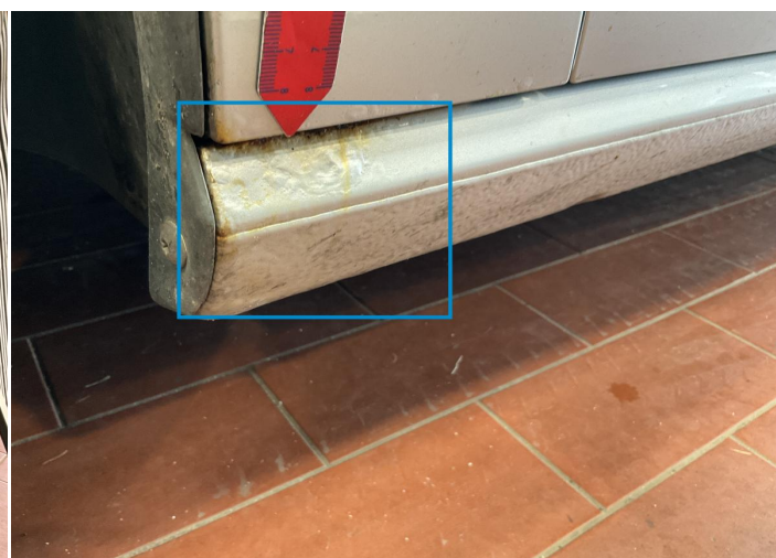
4. Rocker Panel / Center Left Paint / Scratch / Line -
