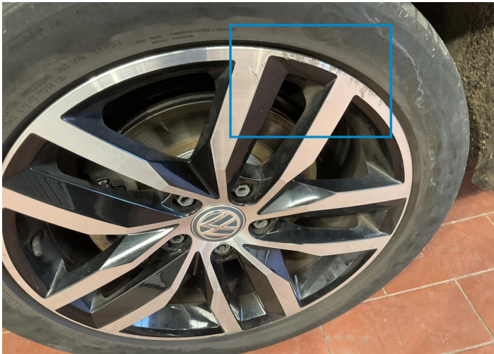
4. Rim / Front Left Out of Bodywork / Scratch -
