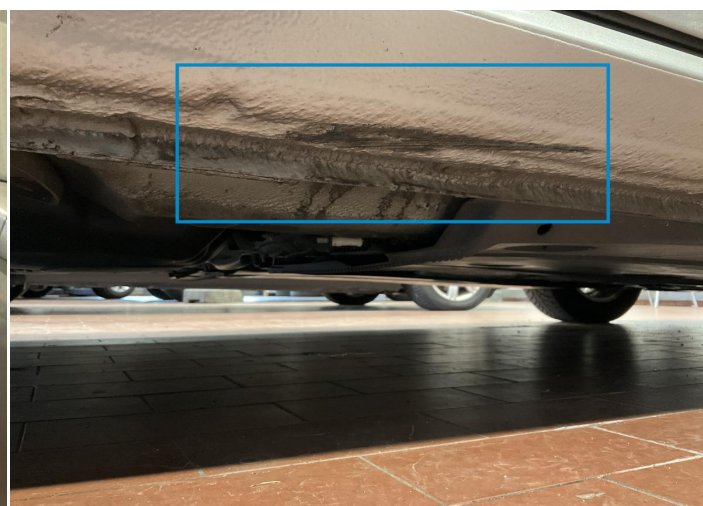
10. Rocker Panel / Center Right Paint / Scratch / Scuff -
