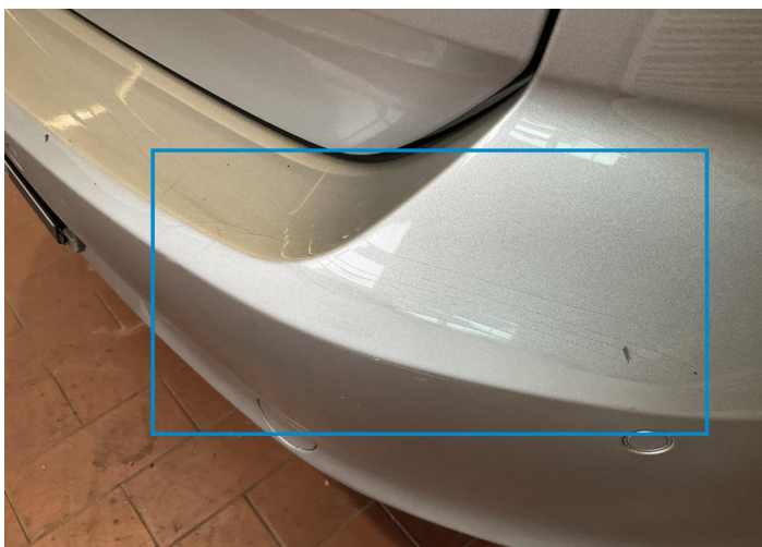
7. Bumper / Back Bodywork / Dent / Dent -
