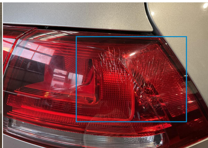
8. Back Light / Right Glass Break / Impact -
