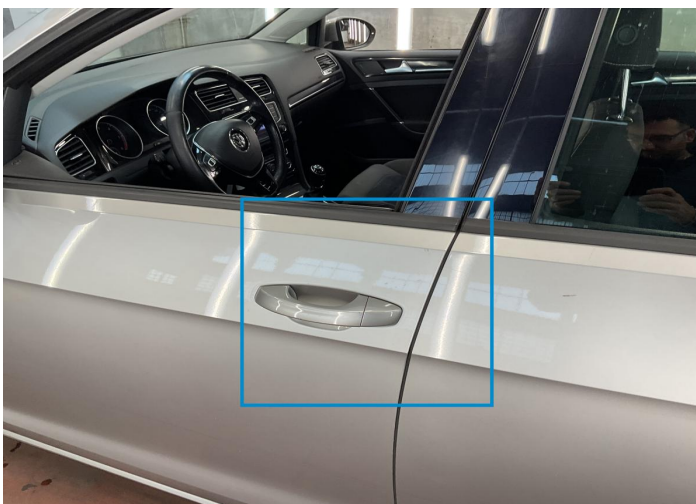
15. Door / Front Left Paint / Scratch / Line -
