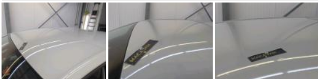
Roof, Chemical polution, Polish
