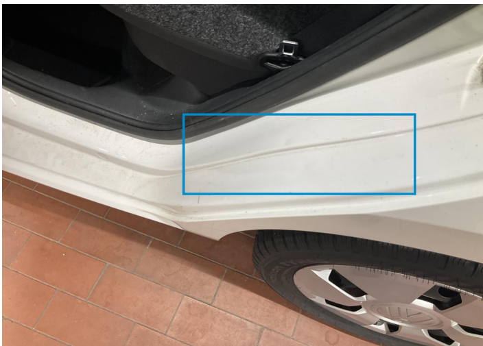
6. Pillar / Back Left Bodywork / Dent / Dent -
