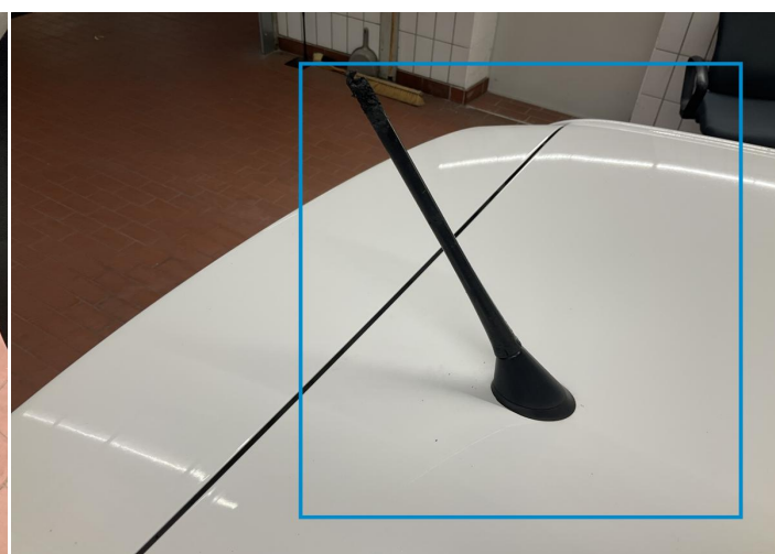
12. Antenna Rod Out of Bodywork / Breakage -
