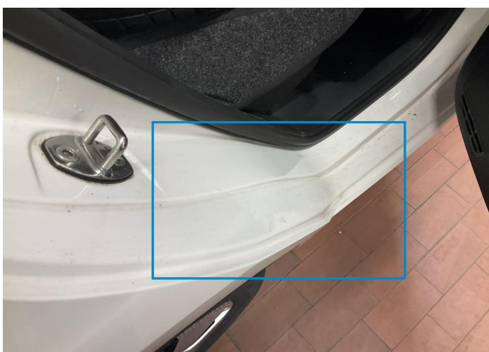
11. Side Panel / Back Right Bodywork / Dent / Dent -
