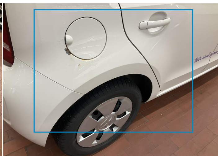
10. Side Panel / Back Right Paint / Corrosion -
