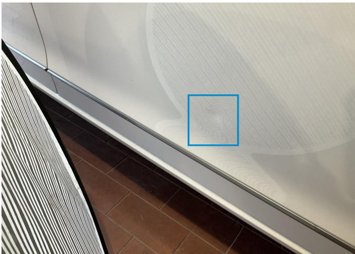
8. Door / Back Right Bodywork / Dent / Dent -
