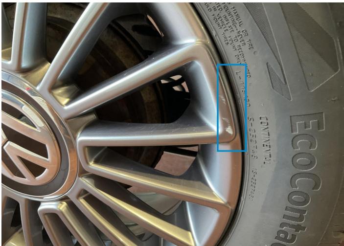
7. Rim / Back Right Paint / Stone Chip -
