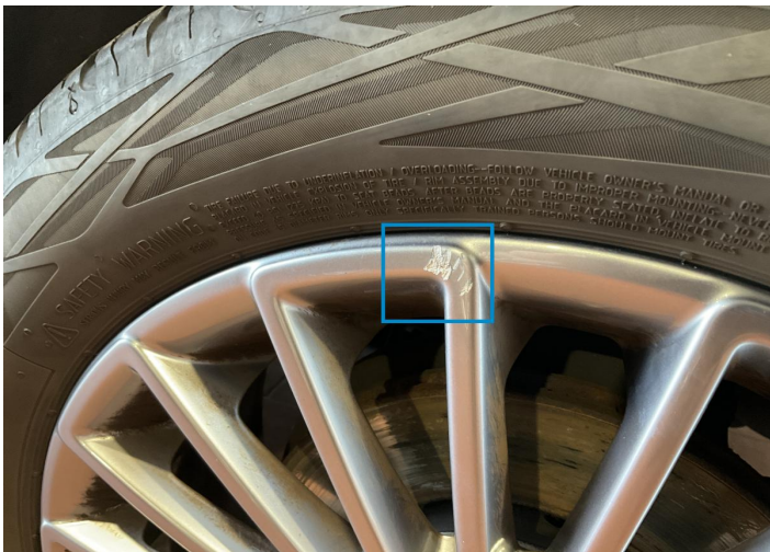
10. Rim / Front Right Paint / Stone Chip -
