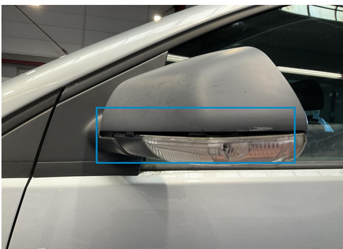
4. Mirror / Front Left Bodywork / Breakage / Crack -
