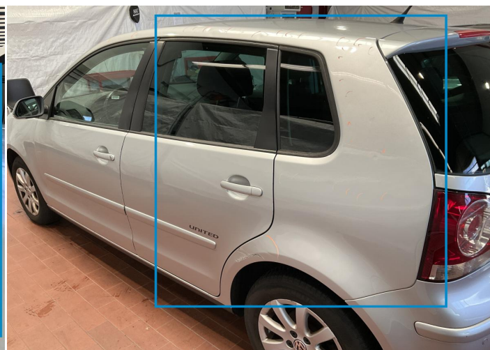
8. Fender / Back Left Bodywork / Dent / Hail Area -
