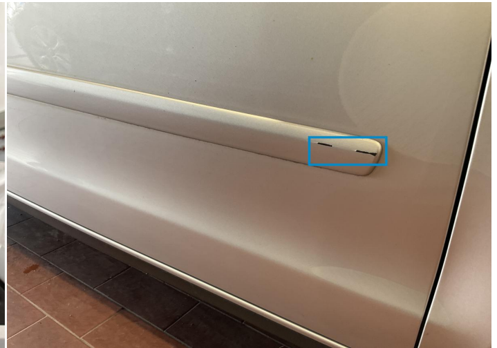
14. Door Side Molding / Front Right Paint / Scratch / Scuff -
