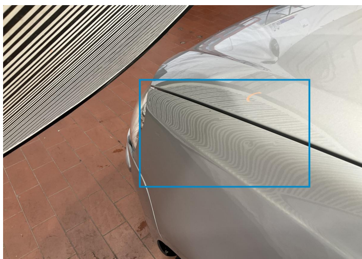
3. Fender / Front Left Bodywork / Dent / Dent -
