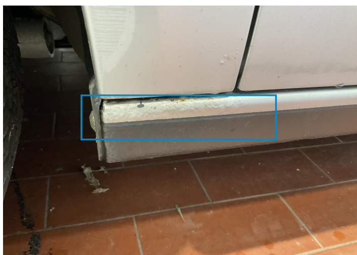
5. Rocker Panel / Center Left Paint / Scratch / Line -
