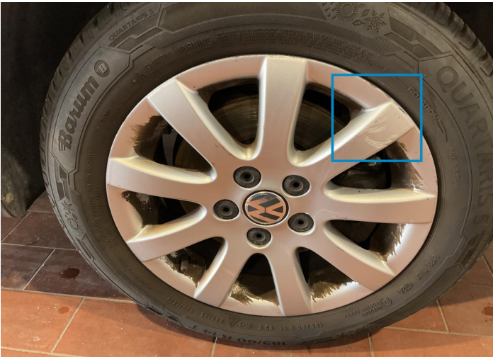
15. Rim / Front Right Out of Bodywork / Scratch -
