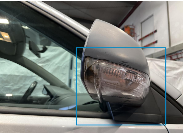
13. Mirror / Front Right Bodywork / Breakage / Crack -
