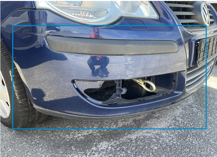
1. Bumper / Front Missing Part -
