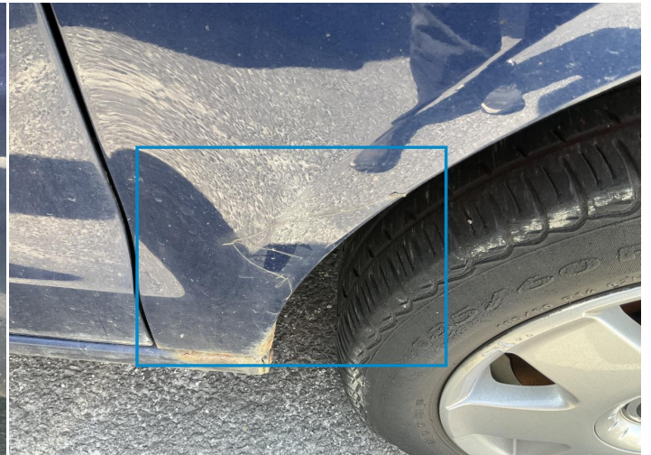
10. Fender / Front Right Paint / Scratch / Scuff -
