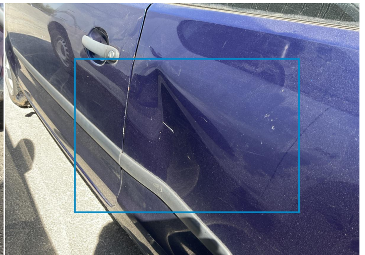
6. Side Panel / Back Left Bodywork / Dent / Dent -
