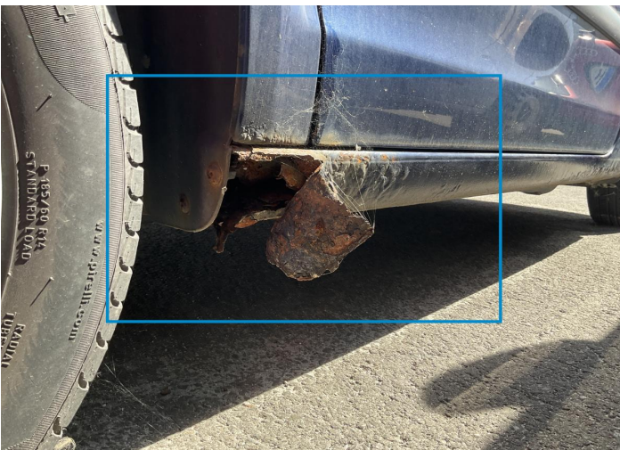
5. Rocker Panel / Center Left Paint / Corrosion -
