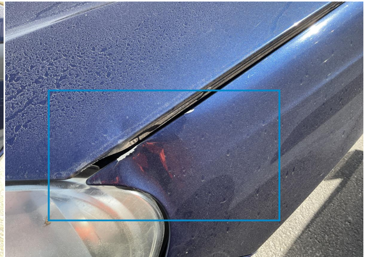
4. Fender / Front Left Bodywork / Dent / Dent -
