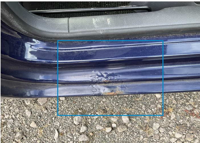
2. Rocker Panel / Center Right Paint / Corrosion -
