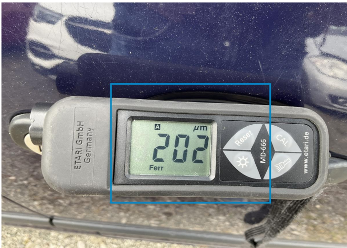
1. Door / Front Right Paint / Poor Previous Repair -
