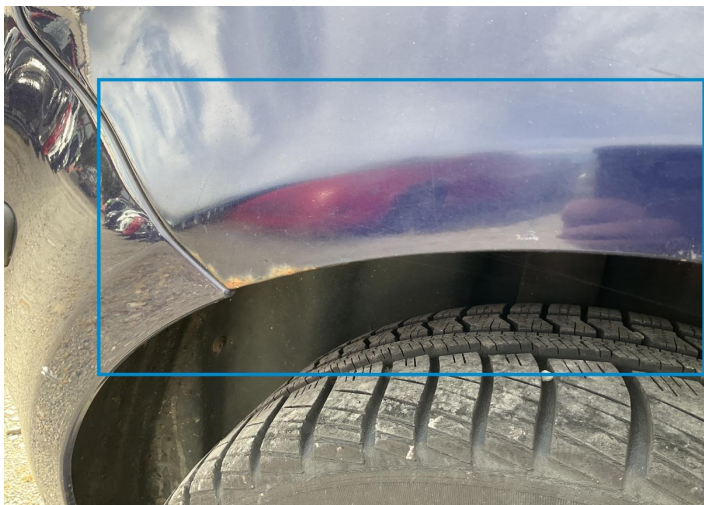
11. Fender / Back Right Paint / Corrosion -
