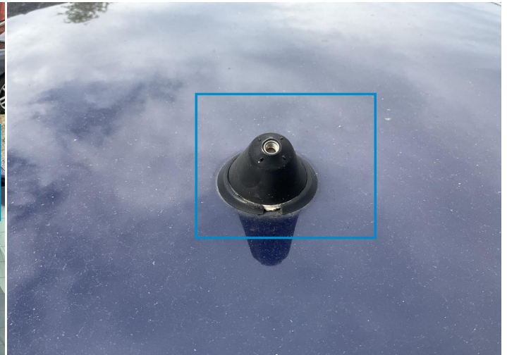
20. Antenna Rod Missing Part -
