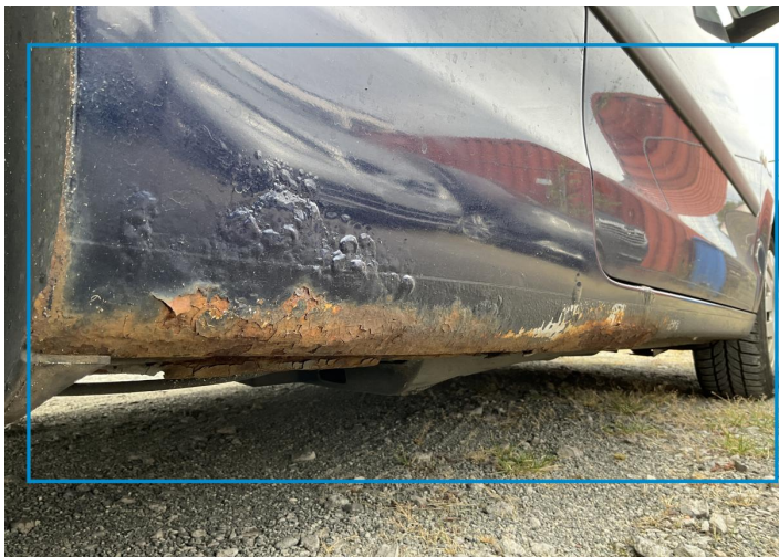
9. Rocker Panel / Center Right Paint / Corrosion -
