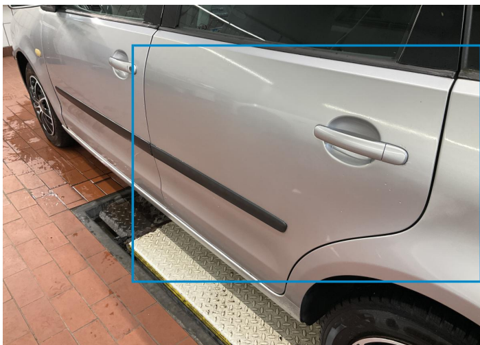
15. Door / Back Left Paint / Scratch / Scuff -
