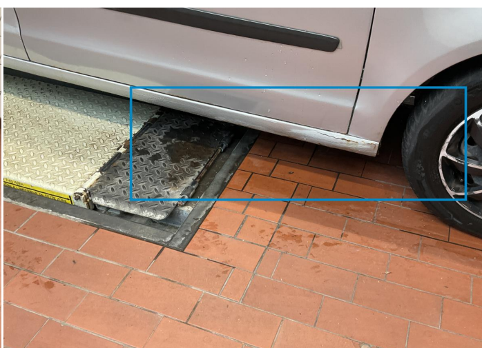
24. Rocker Panel / Center Right Paint / Corrosion -
