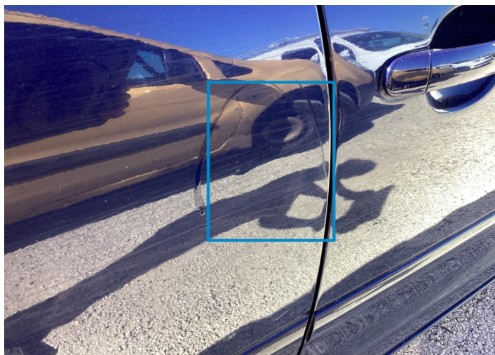
40. Door / Back Right Bodywork / Dent / Deformation -
