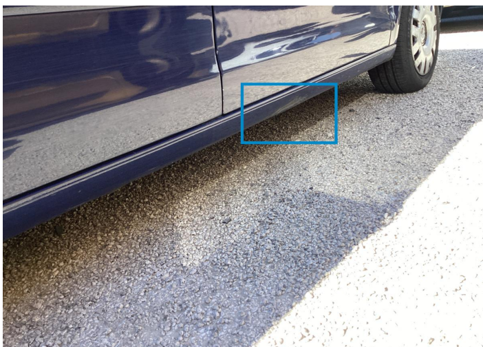
44. Rocker Panel / Center Right Bodywork / Dent / Deformation -
