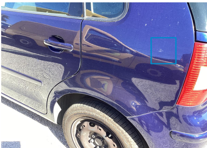
12. Fender / Back Left Bodywork / Dent / Dent -
