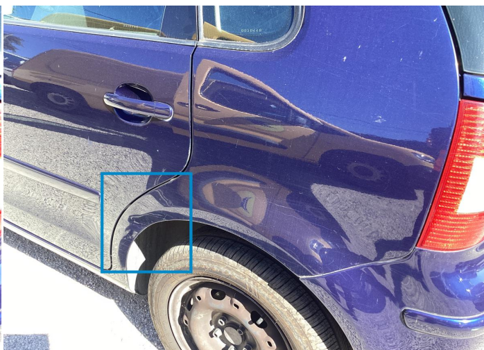
13. Fender / Back Left Bodywork / Dent / Deformation -
