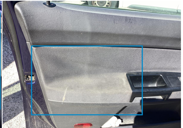
27. Panel Filling / Front Left Interior / Loose -
