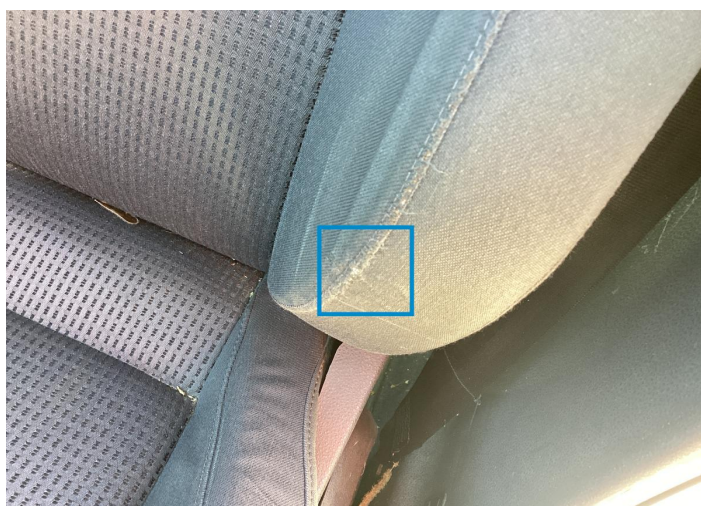
22. Backrest Cover / Front Left Interior / Ripped -
