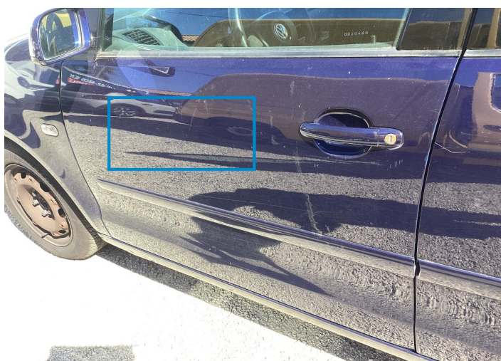
18. Door / Front Left Bodywork / Dent / Dent -
