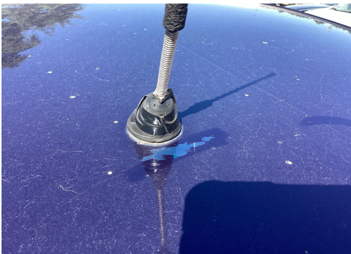
47. Roof Paint / Poor Previous Repair -
