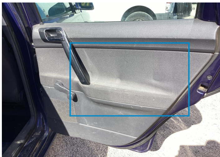
42. Panel Filling / Back Right Interior / Loose -
