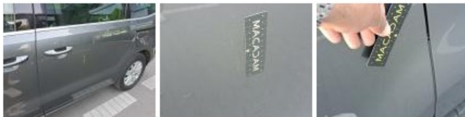
Door seal RL, Deformed / Strained, Replace
