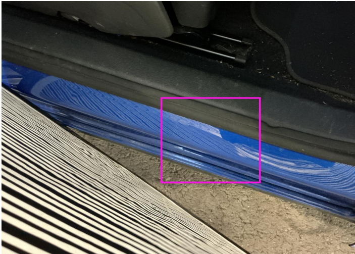
5. Pillar / Back Right Bodywork / Dent / Dent -
