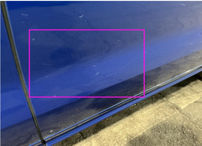
13. Door Slide / Left Paint / Scratch / Scuff -
