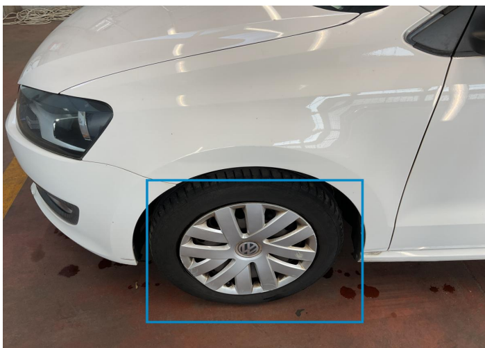
25. Hubcap / Front Left Out of Bodywork / Deformation -
