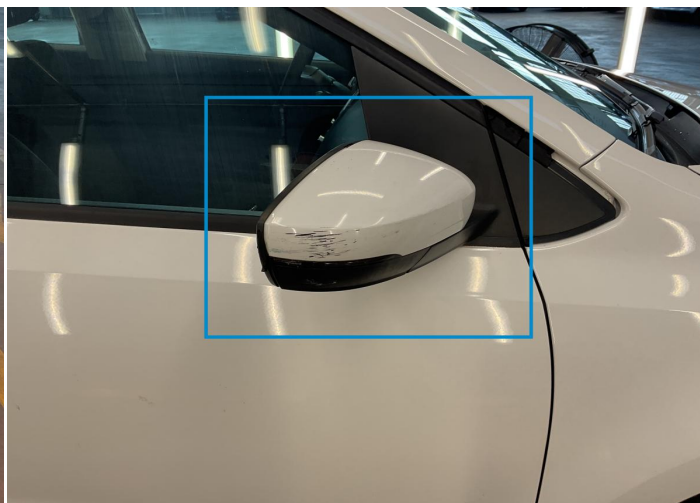
16. Mirror Shell / Front Right Bodywork / Breakage -
