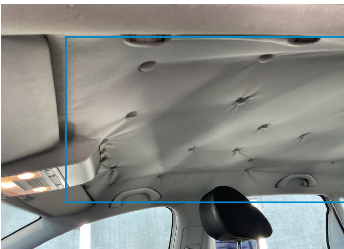
12. Roof Upholstery Interior / Broken -
