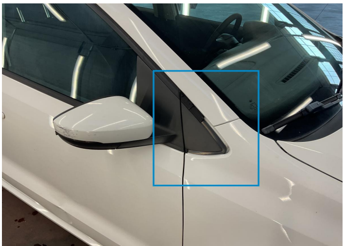
21. Mirror Shell / Front Right Bodywork / Breakage -
