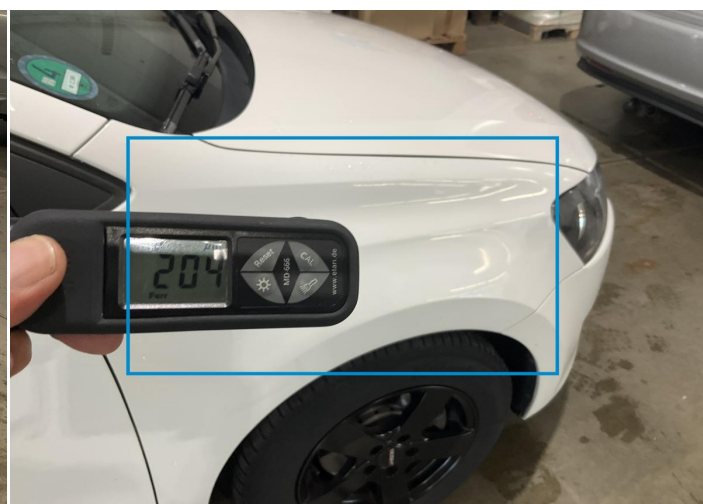
14. Fender / Front Right Paint / Poor Previous Repair -
