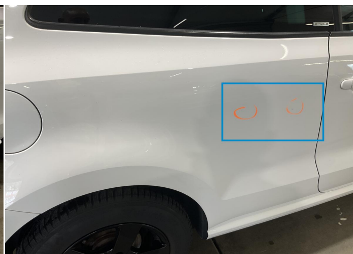
16. Side Panel / Back Right Bodywork / Dent / Dent -
