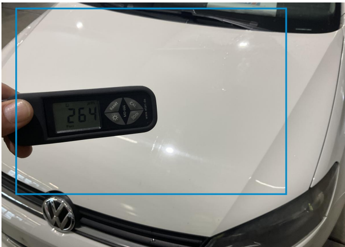
2. Hood Paint / Poor Previous Repair -
