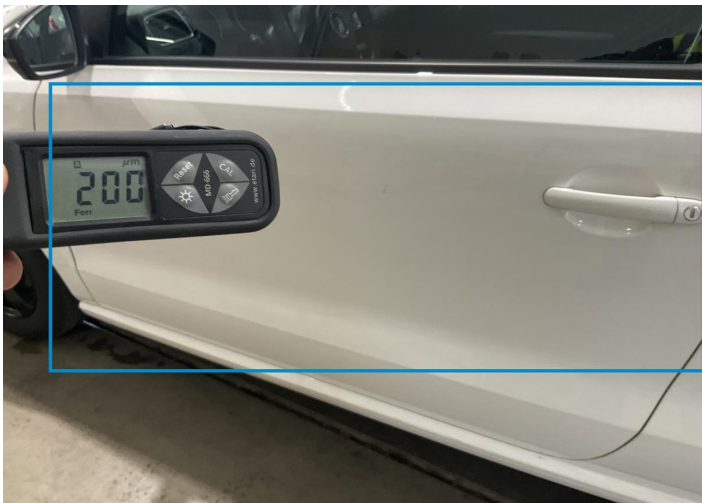
8. Door / Front Left Paint / Poor Previous Repair -
