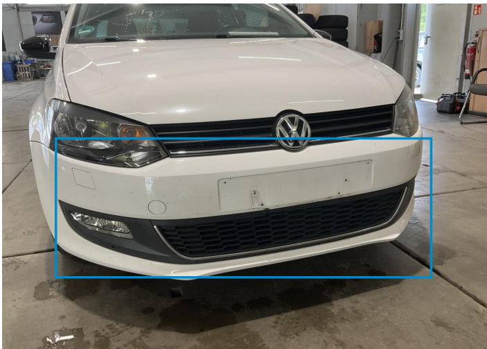
1. Bumper / Front Paint / Stone Chip -
