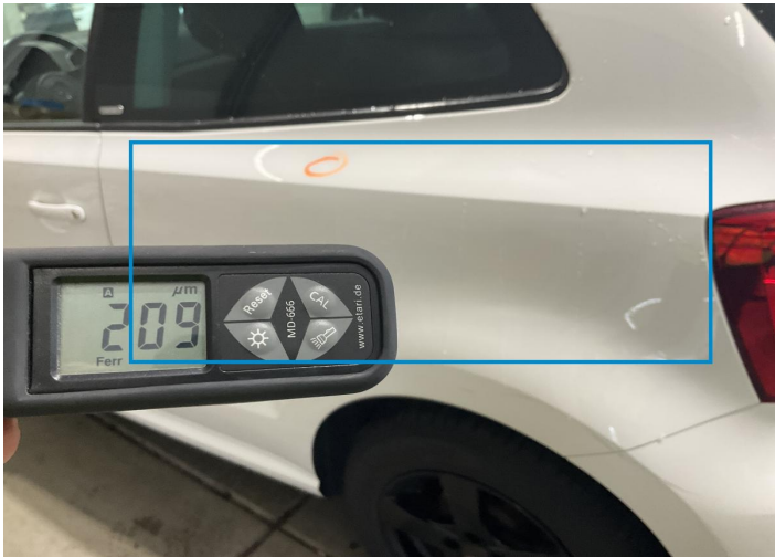
10. Side Panel / Back Left Paint / Poor Previous Repair -
