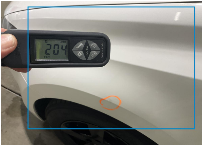
6. Fender / Front Left Paint / Poor Previous Repair -
